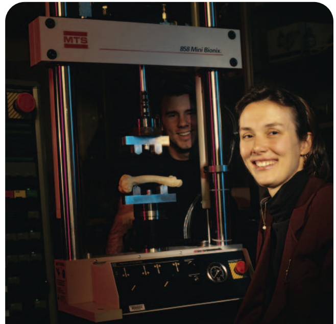
Dr. Marjolein van der Meulen (right) and her colleagues put bones and implants in the 858 Mini Bionix to test their behavior under different load conditions. The student in the photo is now a design engineer at the Hospital for Special Surgery.
